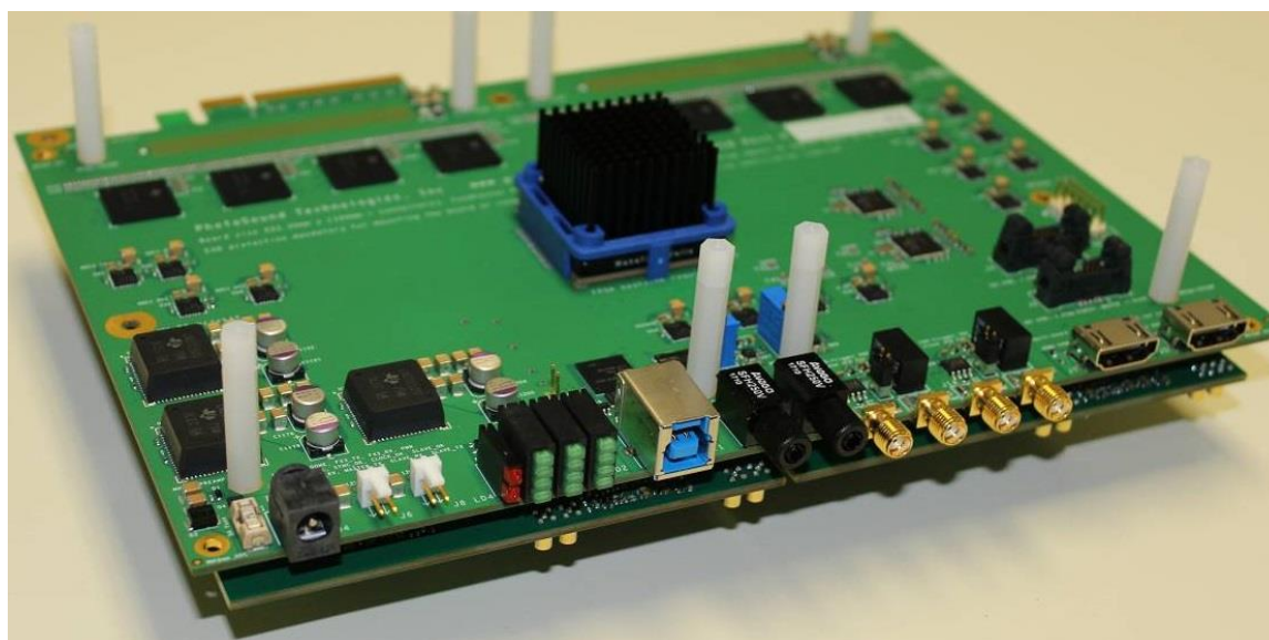
Figure 1: LEGION DAQ256 with ADC256 Rev1.0 board on top. ADC256 front components / connectors from the left-to-right are nano-fuse, power, 2x fans, 4x LEDs blocks, USB3 type-B, 2x optical fiber trigger inputs, 4x SMA trigger IO, 2x HDMI master and slave.
