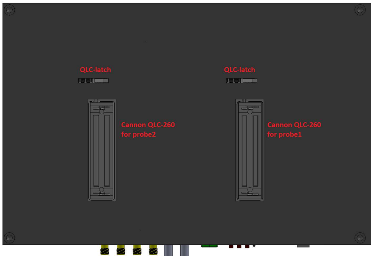
Figure 2: LEGION DAQ256 top (probe connector side) view. Note: probe connector might be different. Note: MMCX test preamplifier IO connectors (not connected to ADC analog interface) might be available on some preamplifier boards. If extra test preamplifier channels are needed order Flash AMP16-18 with SMA interface and optional SMA128 breakout board for ADC256/128.
